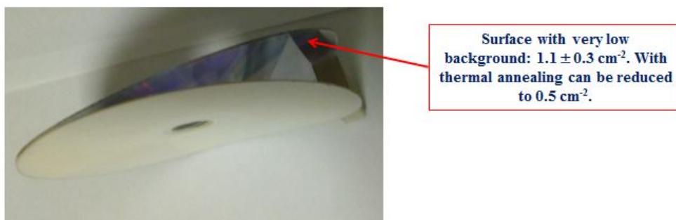
Figure 24- The structure of a DVD: it consists of two halves stuck together. The front half is made of polycarbonate which can be used as alpha-track detector. The background of the internal polycarbonate surface is very low and can be additionally reduced by thermal annealing.
